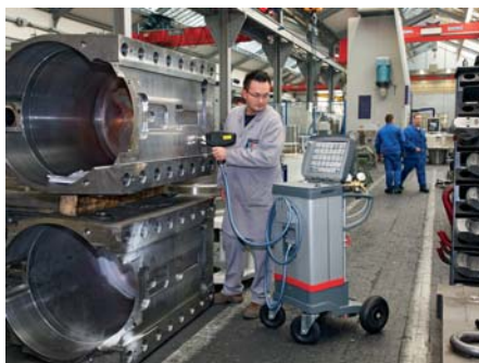
Mobiler Metallanalysator SPECTROTEST
